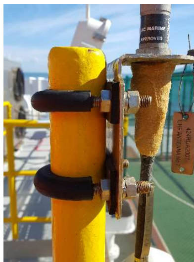
Figure 2: Insulation to avoid galvanic corrosion.
